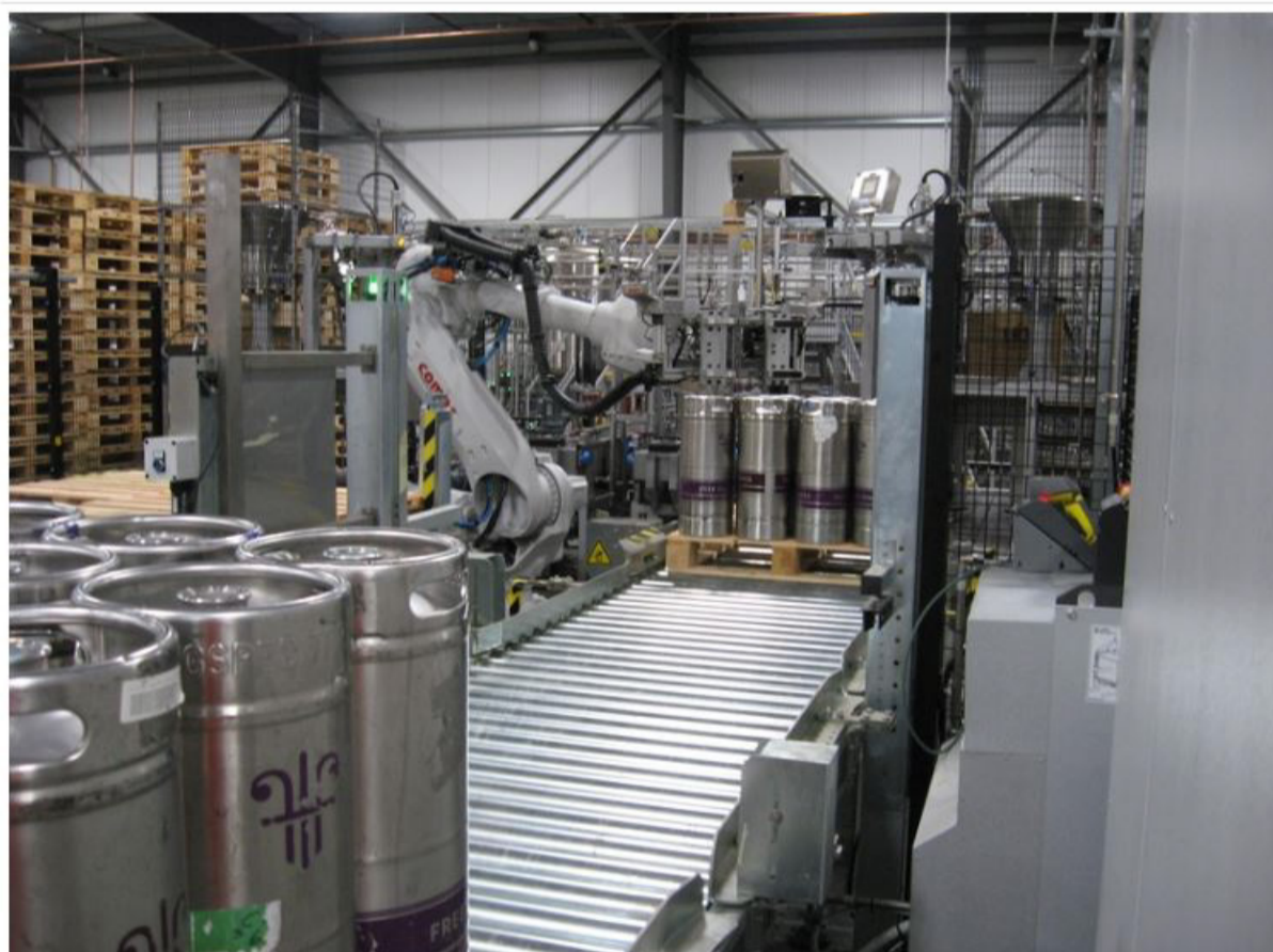
A robot arm moves kegs for cleaning and filling operations in the new Free Flow facility in Sonoma, Calif.
