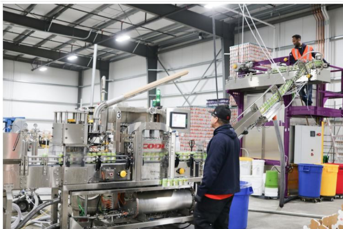
Workers manage one of three current can fillers at the new Free Flow facility, and a fourth filling line has been ordered. (submitted photo)
